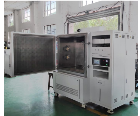
Negative Pressure Test Chamber
